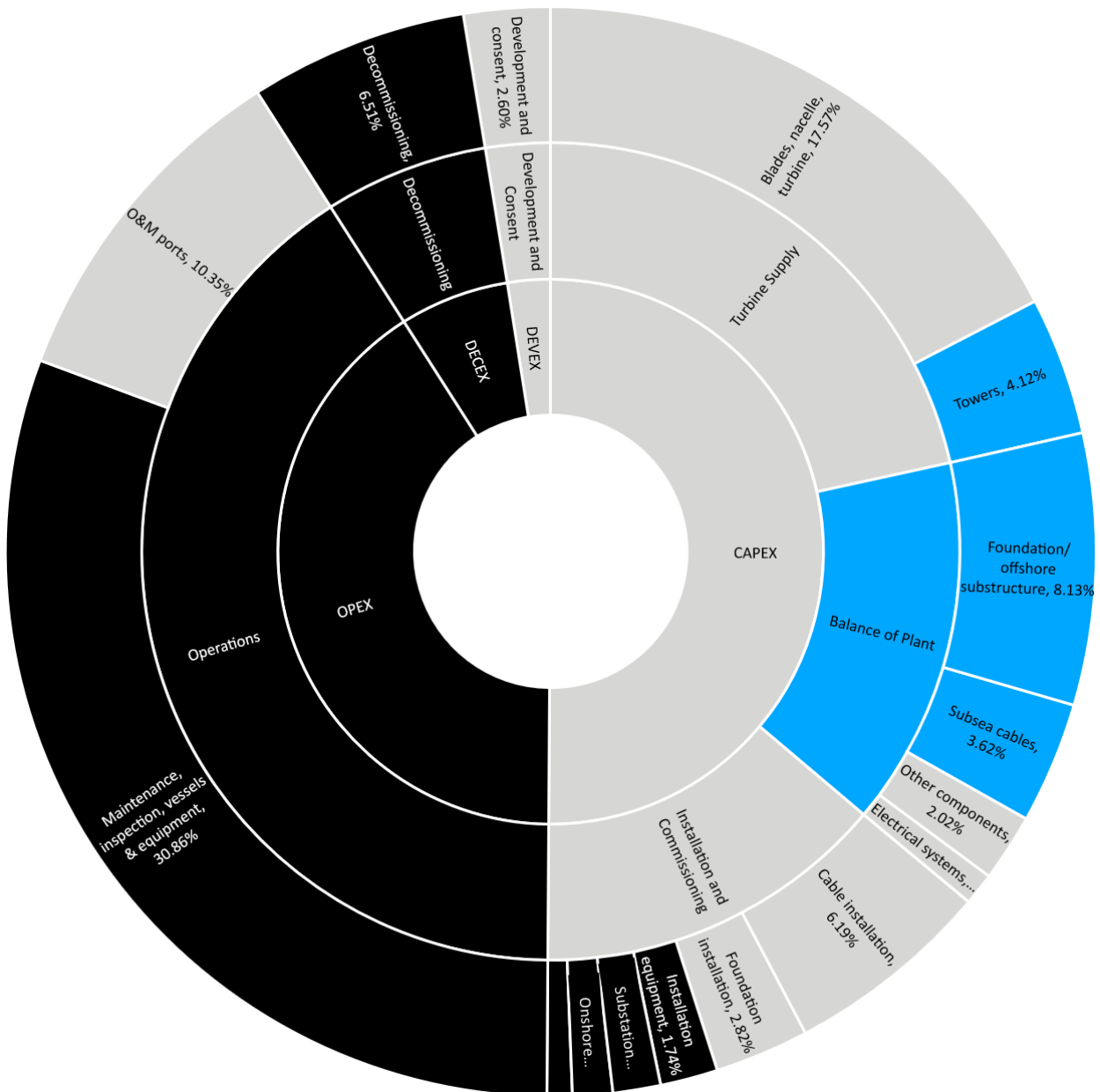
Figure 10: Current supply in South Korea (percentage values show typical cost breakdown for an OSW project). Blue = high, Grey = medium, Black = low.
